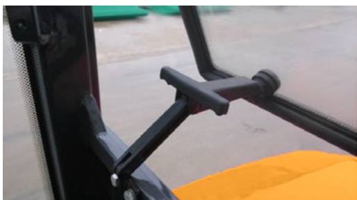
Push both handles at the same time, to open the rear window
